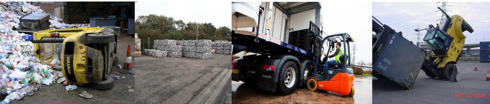
FLT (forklift truck) fall-over during loading of loose wastes, bales awaiting loading, loading a curtain-sided lorry, large FLT fall-forward during loading of a waste container onto rail
