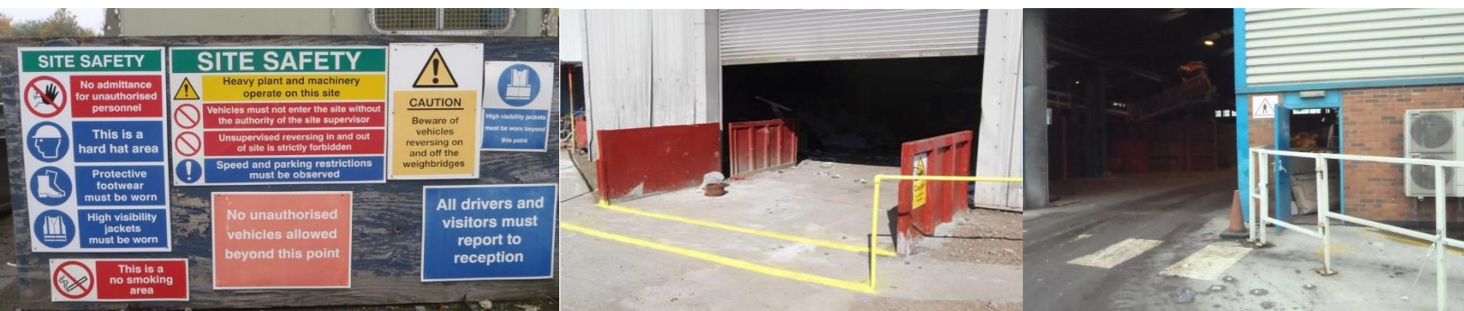
Example of a 'forest of signs' which are unlikely to be fully read by drivers etc, examples of pedestrian control measures at vehicle access/exit doors
