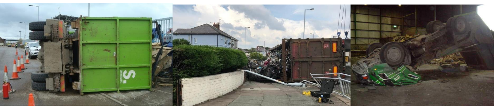
Two examples of waste lorry fall-overs resulting from badly loaded wastes, one on a waste and recycling site and one on the road, and an example ‘flipped’ skip lorry resulting from attempted jogging of a stuck load
