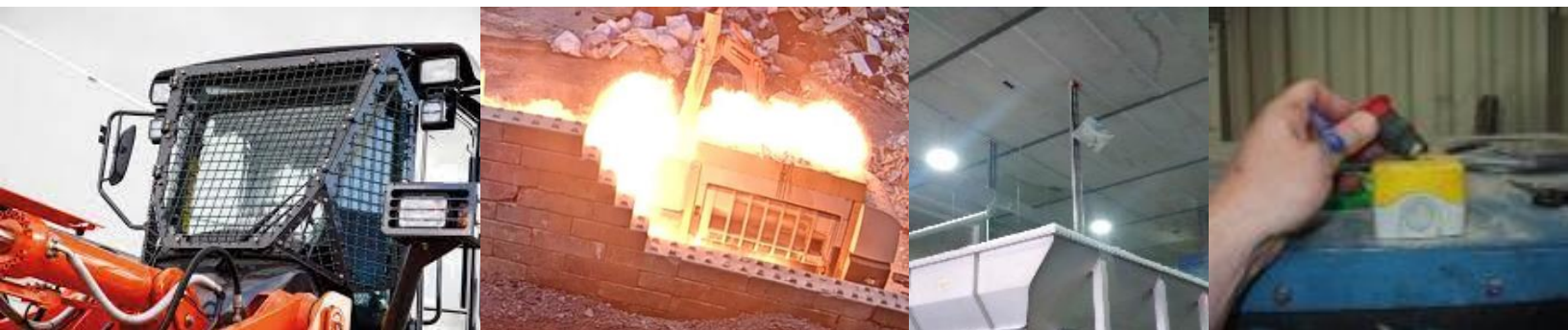
Left to right: trash guard on a loading shovel, fire in a shredder caused by non-conforming flammable materials, mirror above feed hopper to a shredder (see below), damaged emergency stop on a hand-fed shredder (see below)
