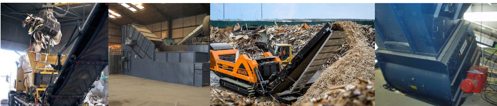
Left to right: shredder being fed by a grab crane, conveyor fed shredder at a recycling plant, moveable/mobile wood shredder, enclosed integrated shredder at a waste recovery plant with conveyor feeds in and out
