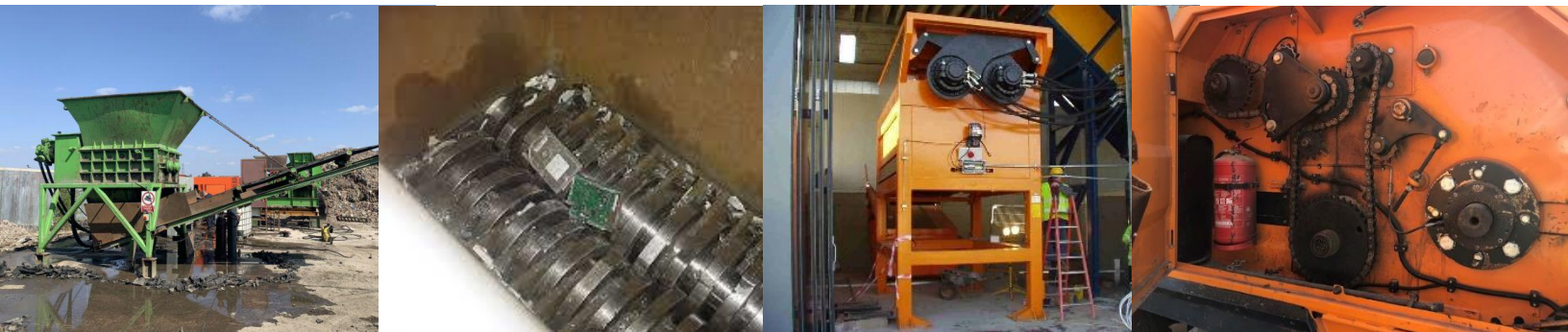
Left to right: tyre shredder fed via a load hopper with output conveyor, twin shredding elements of a computer hard drive shredder, installation of a large twin element shredder at a recycling plant, chain drive on a moveable shredder
