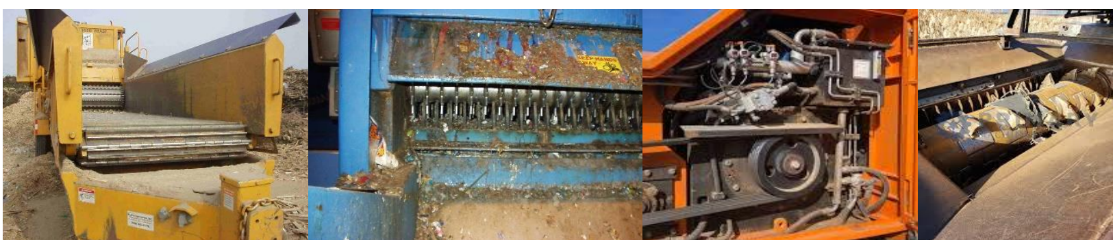
Left to right: example of a (very) badly safeguarded shredder hopper (easy to access), exposed shredder element during cleaning, belt drive on a large moveable shredder, shredder element on a hopper fed shredder
