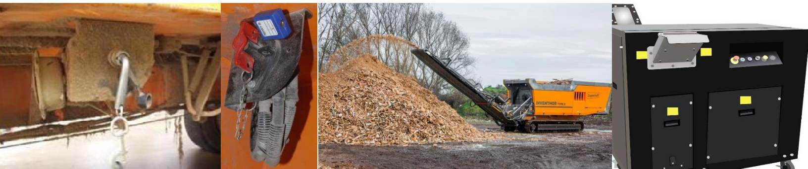
Left to right: two examples of battery isolator switches on the lower/under carriages of shredders, waste wood shredder with output conveyor, small hand-fed IT disc/drive shredder with removable output bins
