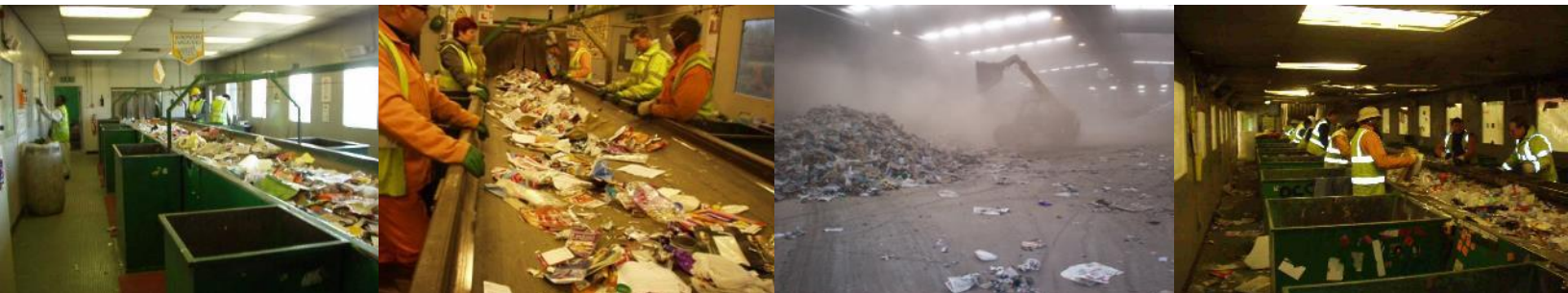
From left, daily clean-down in a MRF picking cabin, typical picking belt in a cabin, dust can be a problem in MRFs (in this case a new and particularly dusty waste stream), picking cabins should be kept clean and free of excessive debris etc, unlike this one – would you want to work here?
