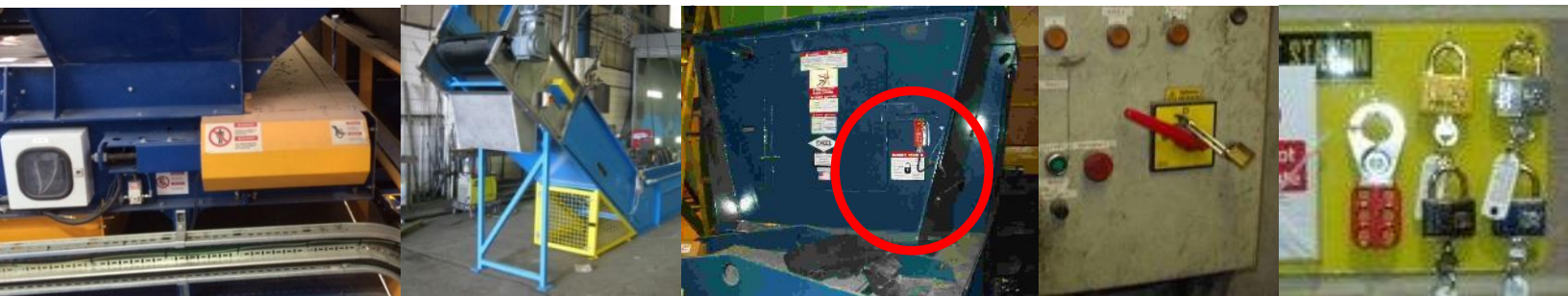
From left, examples of, belt conveyor tail roller guard designed to allow tracking without guard removal, drop-out chute fitted at a feed conveyor aimed at reducing detritus build-up issues, interlocked guard fitted to a baler access hatch, single padlock lock-off at a MRF control panel, lock-off board including individual padlocks and lock-off plate
