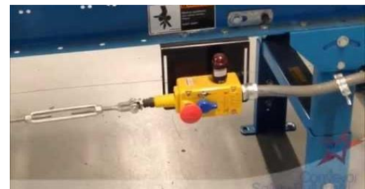
Left to right: Floor mounted load conveyor fitted with a pull-wire emergency stop array (red wires supported on blue goal posts), simplified diagram of a pull-wire array with vertical wires hanging down from the pull-wire so that a person prone on the conveyor can reach them, typical pull-wire activation switch
