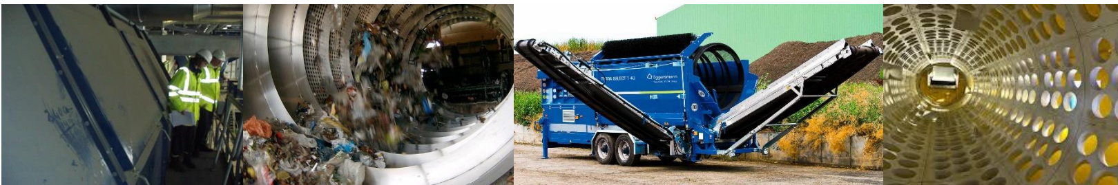
Left to right: large fully enclosed trommel screen with walkway access, interior of a trommel screen, example mobile/transportable trommel screen, interior of a trommel screen during installation
