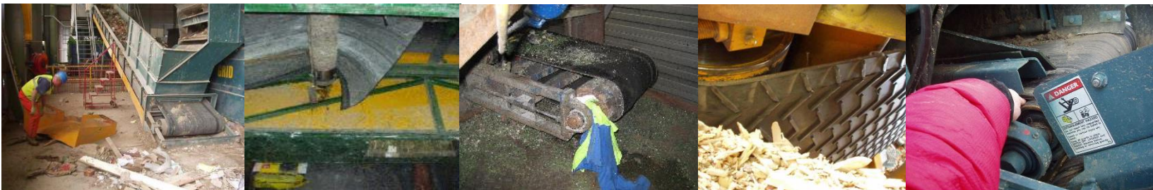
Left to right: tail roller of belt conveyor (guard removed), deflection roller (belt cut to remove injured person), damaged conveyor at and end roller (scene of accident), example in-running nip, second example in-running nip
