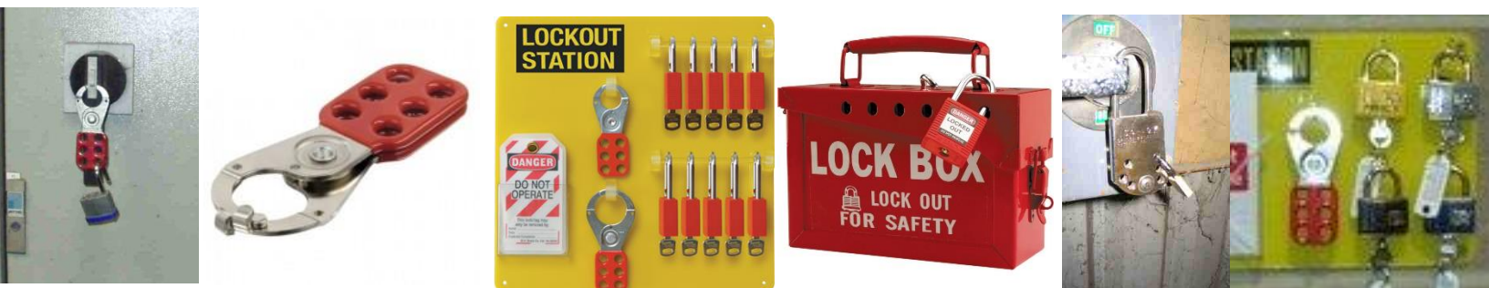
Left to right: A 'crab's claw' lock-off plate in use (only one padlock fitted- open - holes for six locks), crab's claw plate – claw closes through isolation switch and padlocks are inserted – all need to be removed to open the plate, example lock-off station/board, example lock-off box – main key in box and personal padlocks secure the box shut, example alternative type of lock-off plate, another example lock-off station/board
