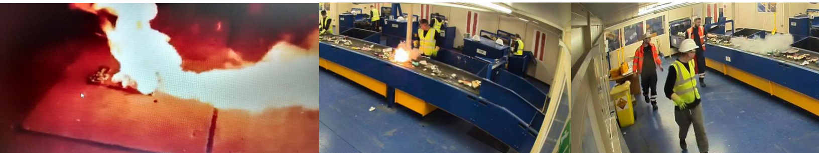
Left to right: Flame jets from a waste lithium battery from a portable computing device discovered at a waste recycling site, CCTV stills showing ignition of a lithium battery from a hand-held power drill in the picking cabin of a recycling plant
