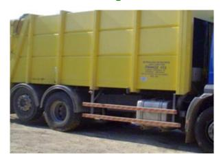
Fitted to large vehicles where the wheel height presents significant risk of cyclists, other two wheeled road users, small cars and pedestrians, travelling, or being drawn under the vehicle bed.
