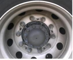
Various types of aid available, such as: Yellow indicators which show that a wheel nut has loosened when one of the points does not line up with its partner, or RIC clips which hold nuts secure by interlocking against each other.
