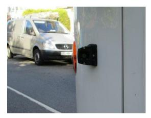
Rear View: Gives view from the rear of the vehicle and to the corner side (depending upon camera type). Used for confirming the danger area of bin lift and the rear of the vehicle is clear of operators, pedestrians or vehicles. Normally used alongside an audible reverse warning alarm.
