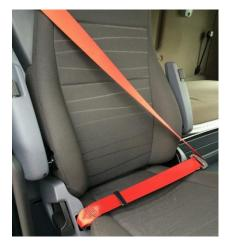
High Visibility seat belts and sheaths cover seat belts in high visibility colours making their mandatory wear easier to monitor and inspect from the roadside.
