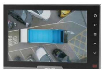
360 Vision: As above, with the addition of a forward view camera (4 cameras in total) giving all round (360 degree) vision) from the vehicle cab, this can also be coupled with an alarm to warn operators if hazards are present. These cameras may be of particular use in urban areas with heavy cyclist and pedestrian presence.
