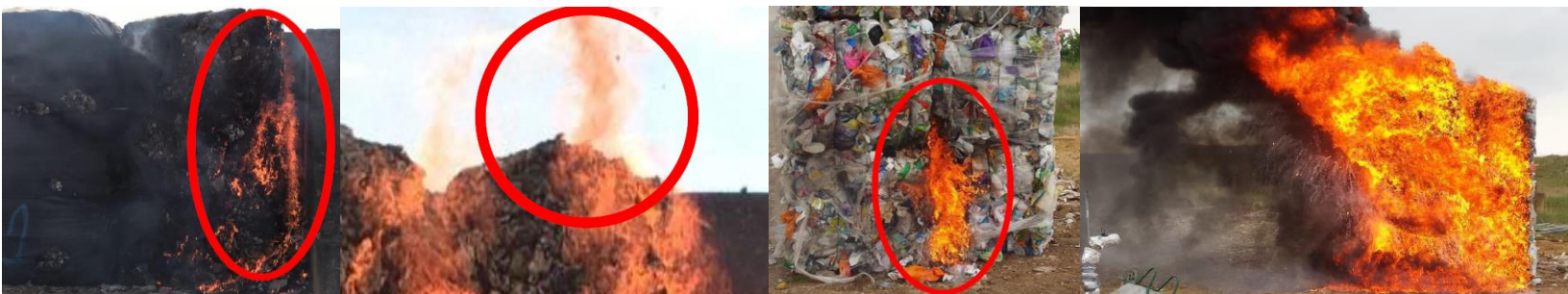
From left: Development of fire vortex behaviour during bale burn tests, visible fire vortex at top of gap between bales during bale tests, development of fire spread in gaps between bales, leading rapidly to a fully developed fire (see bale comments above)
