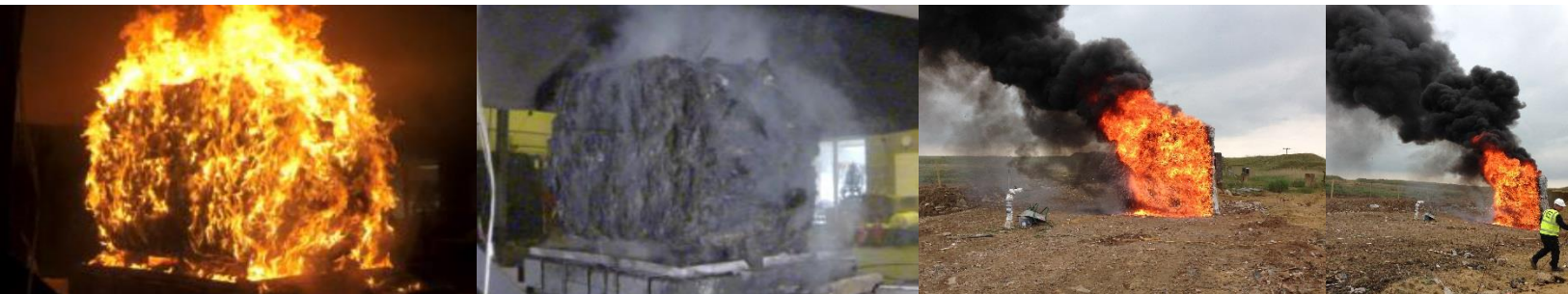
From left: HDPE bale burn during phase 1 smaller scale tests, and same post-burn showing relatively intact bale. Compared to larger scale simulated plastics waste bale stack burns
