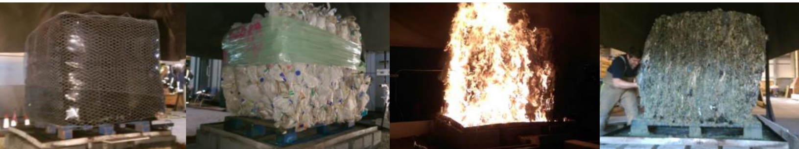
From left: Baled RDF pre-burn, baled LDPE plastic pre-burn, during burn and post-burn (note bale post-burn showing relative lack of fire penetration leaving the bale largely unburnt)
