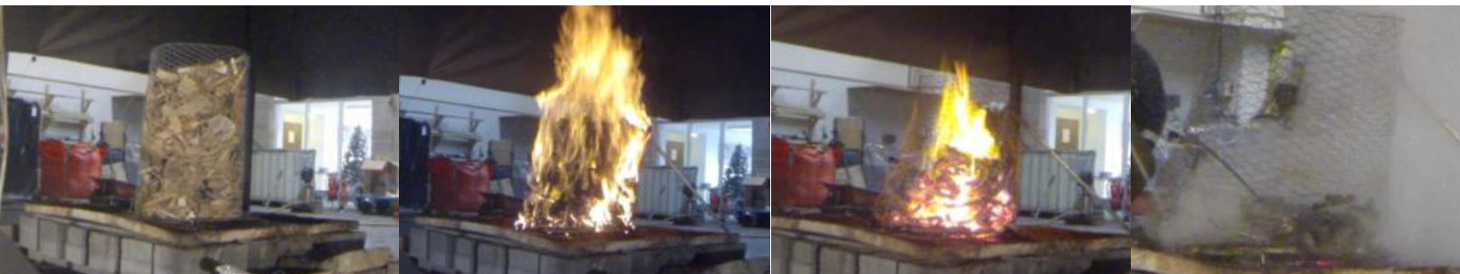
From left: Loose pre-crush wood waste pre-burn (note retained in mesh 'cage'), in initial phases of burn, during steady state burn and post-burn (note much more complete combustion than for baled wastes)
